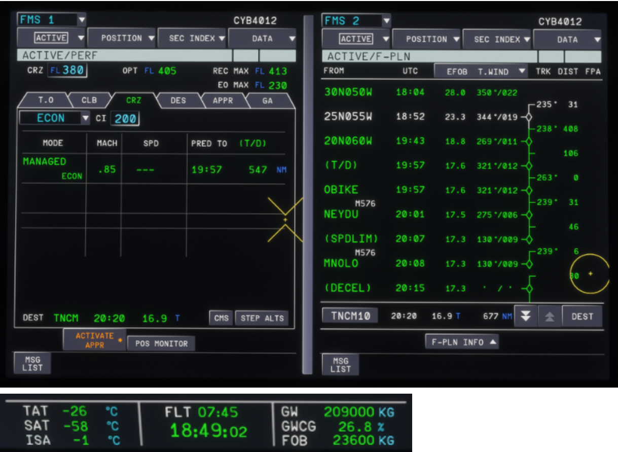
Figure 3. Crops of the pilot's original 18:49 screenshot. The upper aircraft status strip shows 23,600 kg FOB; both FMS destination fields show 16.9 t. The crop is resized but the displayed data are not edited. [4]
